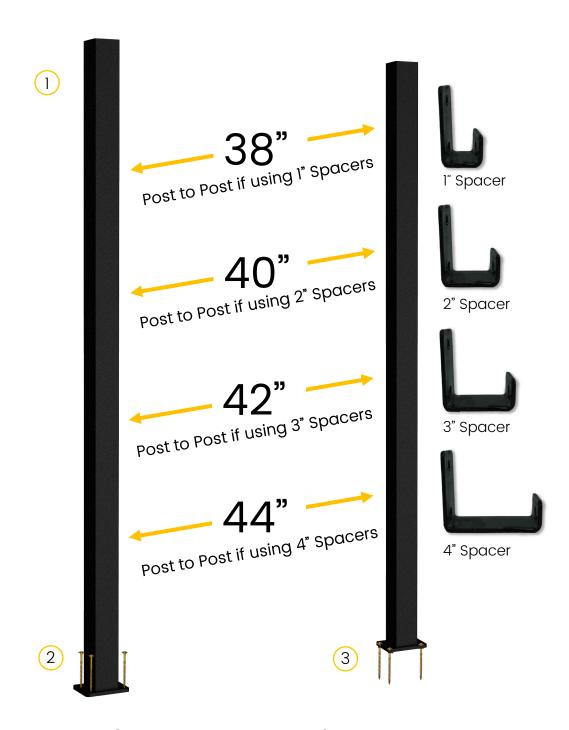
Measuring Post to Post (not base to base), mount Screen Posts 36" apart plus the distance of 2 Spacers being installed.
