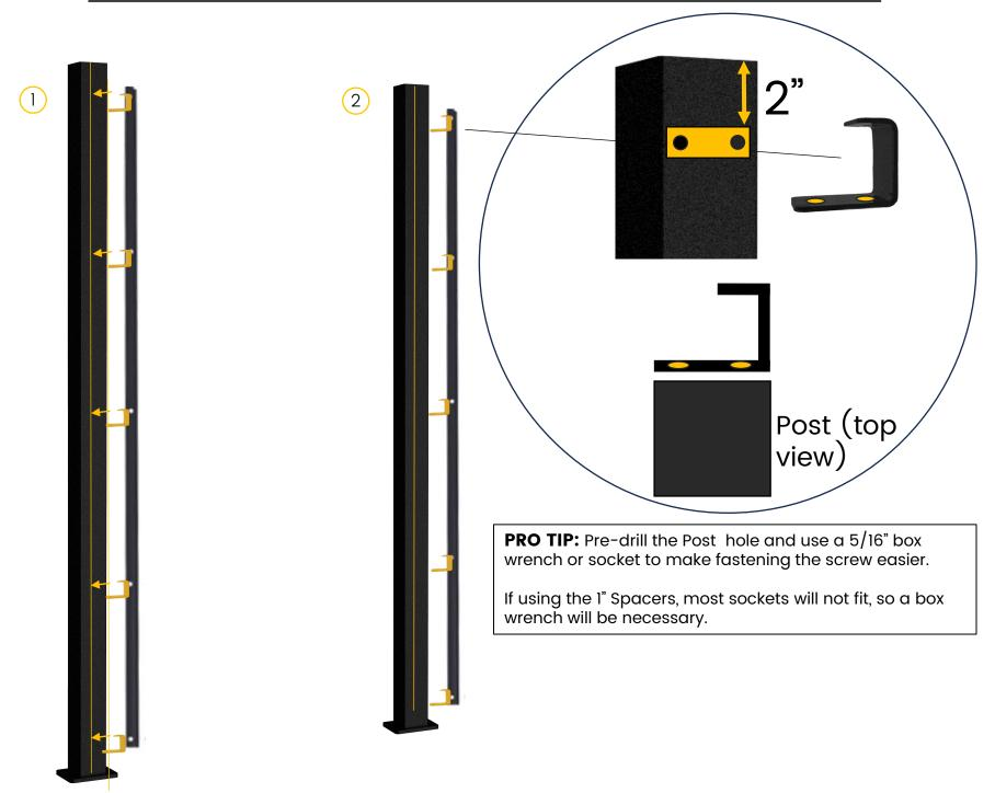
Measure and mark the Post 2" from the top. Line up the top of the Spacer (on the side with 2 holes) to the marked line and center to the Post horizontally. Attach to the Post with 2 self-tapping screws. Continue to center and fasten all Spacers down the length of the Post.
