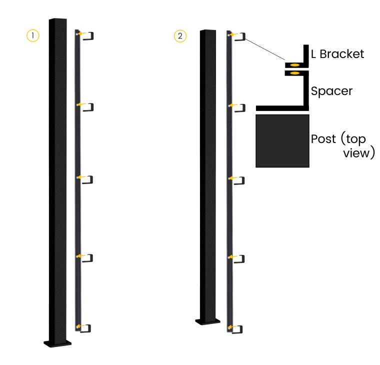
Attach the side of the Spacers with a single hole horizontally to the L Brackets using (5) nuts and bolts per Bracket.
